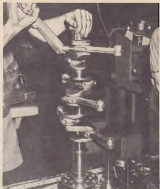
FIG. 47. Torquing Connecting Rod Bolt
