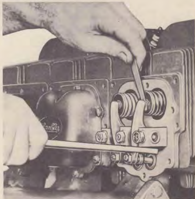
FIG. 49. Checking Valve Clearance
