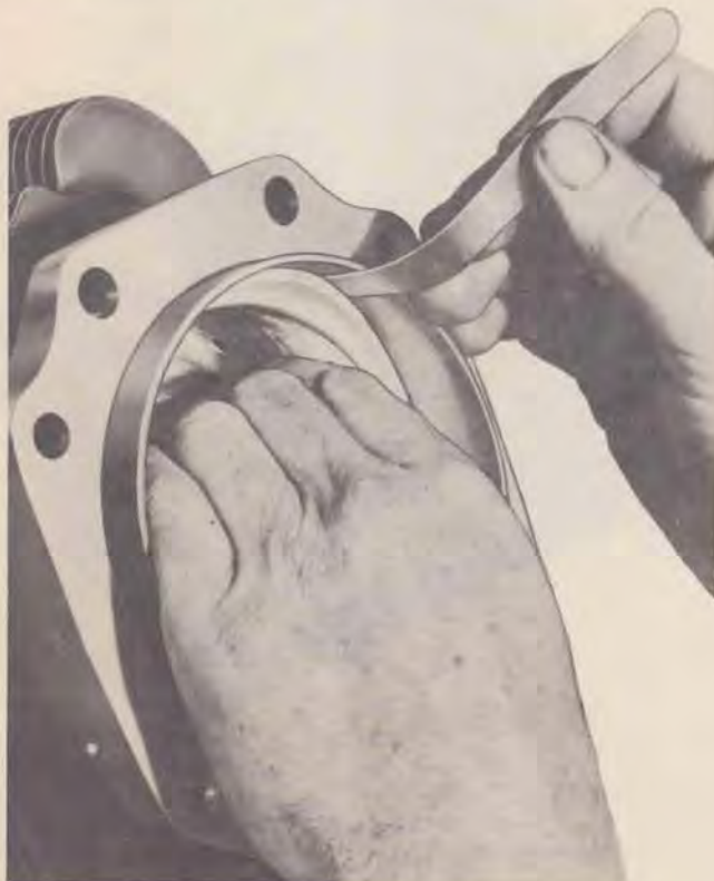
FIG. 10. Checking Piston Clearance
