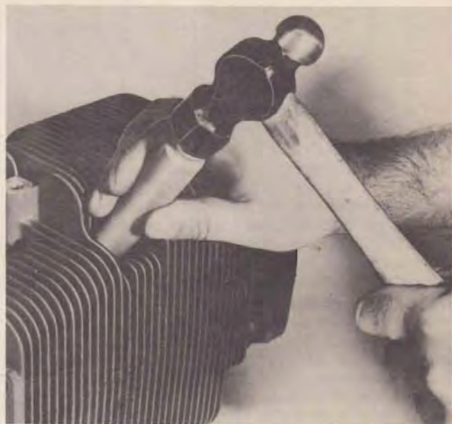
6. Securing the Helicoil in Position
